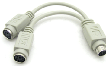
Figure 4-26 Y-Cable use for both Keyboard and Mouse
