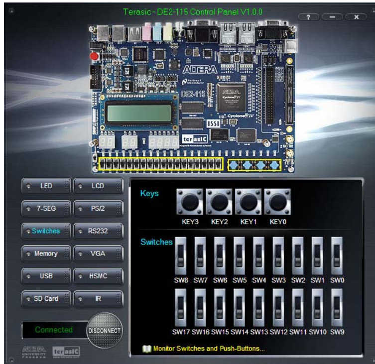
Figure 3-6 Monitoring switches and buttons
