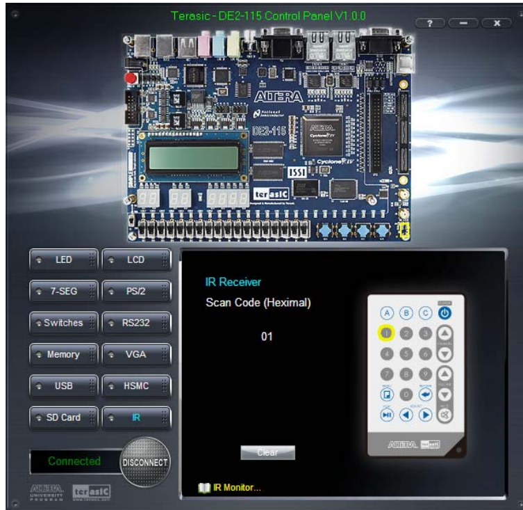
Figure 3-14 Testing the IR receiver using remote controller
